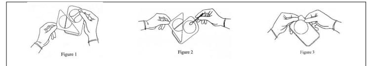
Streak laboratory sample onto the agar surface for isolation (Fig. 2). Reseal the InTray<sup>™</sup> label to the plastic tray body. **Press all around the perimeter of the InTray<sup>™</sup> to ensure a complete seal** (Fig. 3). Immediately label the InTray<sup>™</sup> with sample information and date. **DO NOT COVER THE VIEWING WINDOW.**
